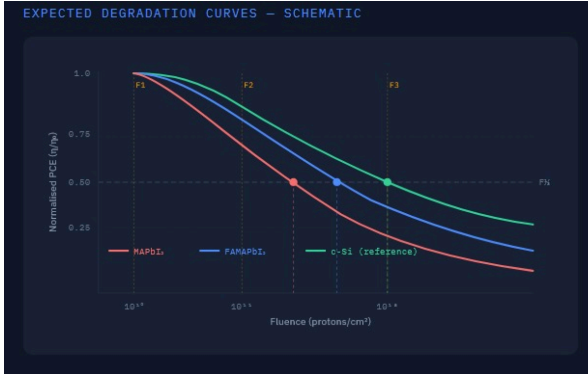
Fig. 3 Expected form of degradation curves; silicon reference validates protocol against established NIEL data [7]
